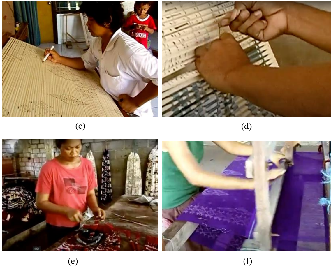
Figure 2. (a) splitting weft threads; (b) transferring weft threads into a frame, (c) drawing pattern on a weft threads frame, (d) tying patterned weft threads frame, (e) coloring weft thread frame, (f) weaving on a non-machine weaving loom
