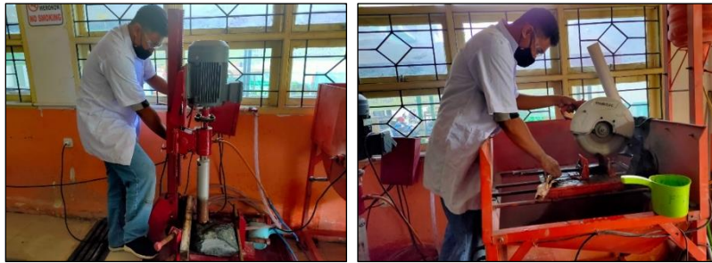
Figure 6. Drilling and cutting of rock sample
