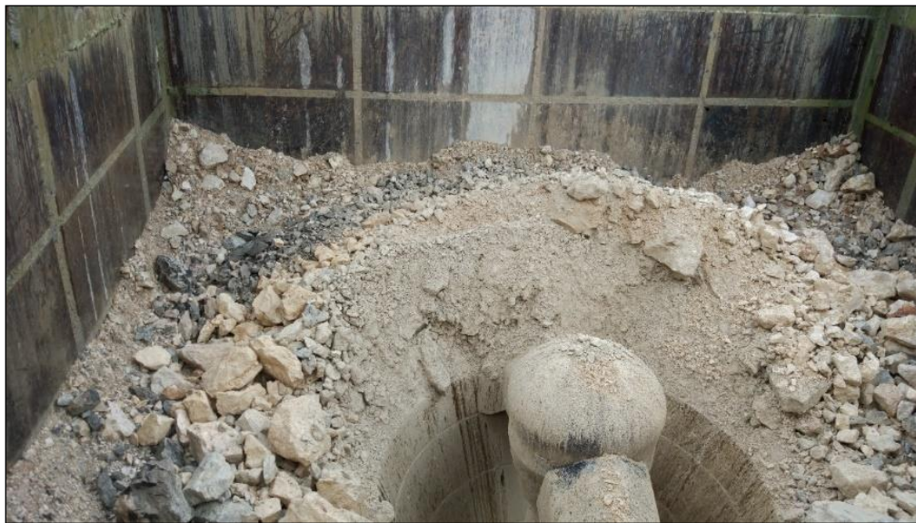
Figure 8. Rock Fractionation in the Hopper Crusher
