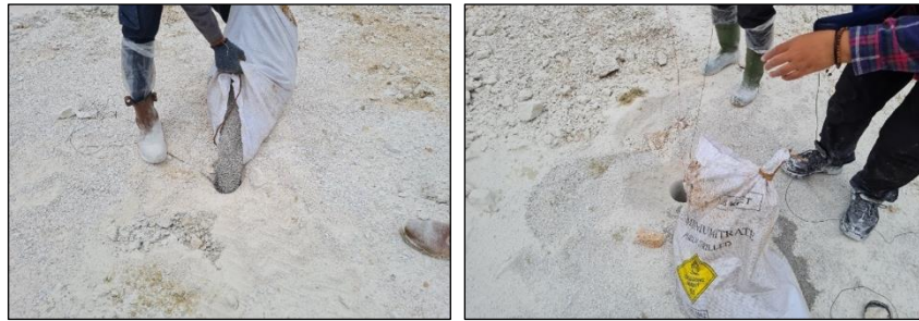
Figure 2. Filling and measuring of explosive contents
