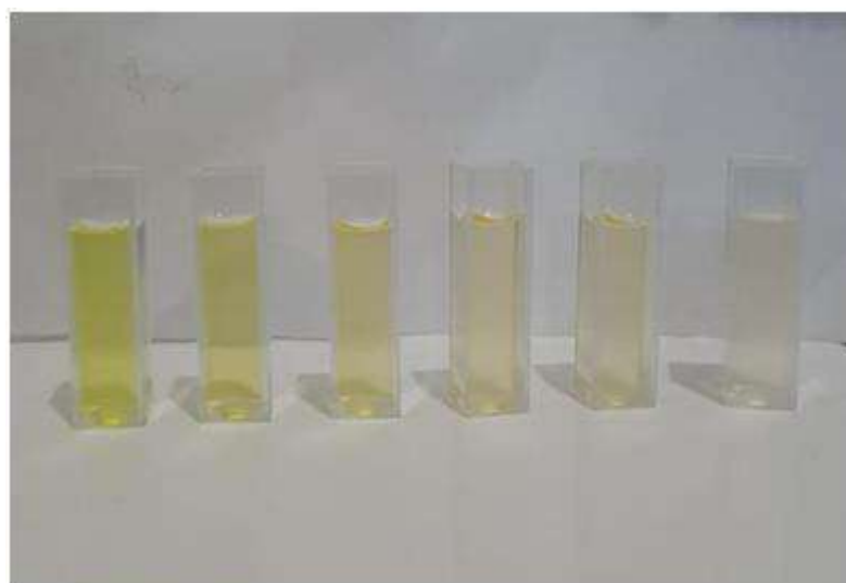
Figure 4 Change in Color of Tartrazine Solution after Irradiation with Dose (from left to right) 0; 0.62 ; 1.24 ; 1.87 ; 2.49 ; 3.11 kGy
