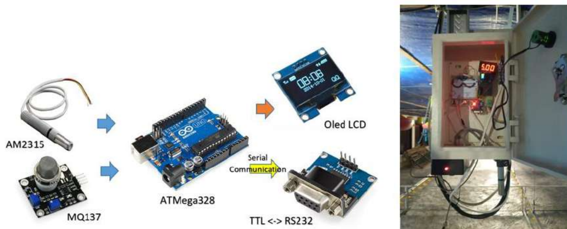
Figure 1. System block diagram of sensor unit
