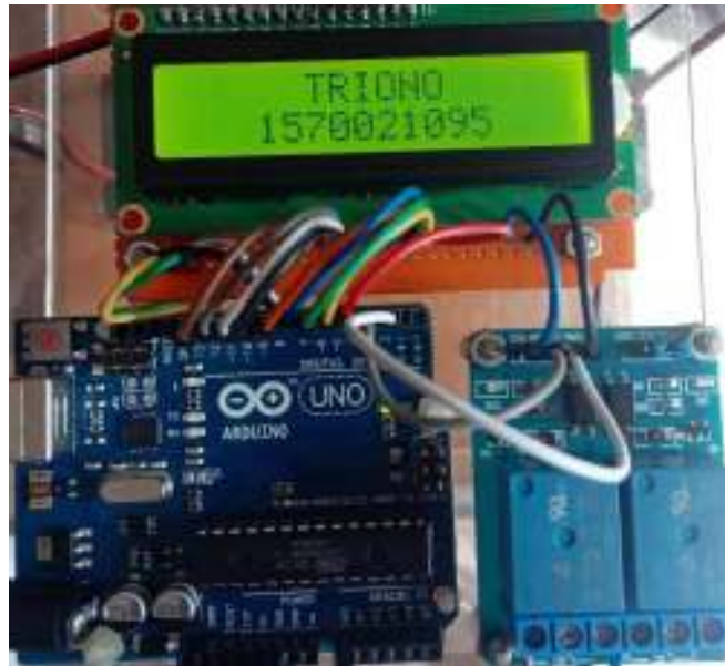
Figure 4. Indoor CO 2 Gas Concentration Control Device
