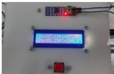
Figure 8. LCD of power per phase and total power.
