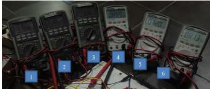
Figure 9. Multimeter as a reference for measuring voltage and current
