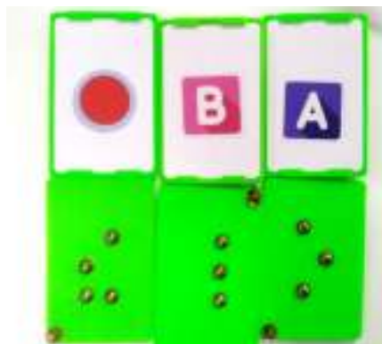
Figure 5. The RFID cards of braille for Braille learning reading aid
