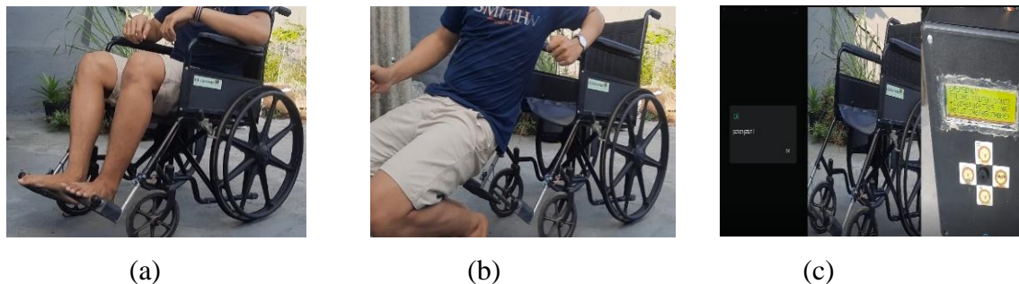
Figure 8. Testing of Ultrasonic and Proximity E18-D80NK Sensors (a) The sensor detects the presence of the user, (b) The user falls down in front of the wheelchair then the sensor can't detect the user, (c) Wemos sends emergency message
