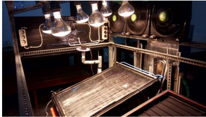
Figure 1. Distillation with fabric and cooler spray
