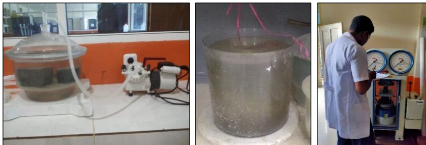
Figure 7. Physical properties and mechanical properties testing (UCS)
