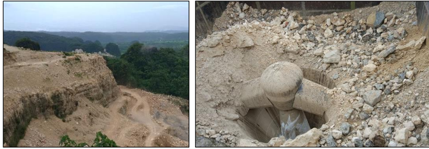
Figure 4. Mining pit and crusher hopper
