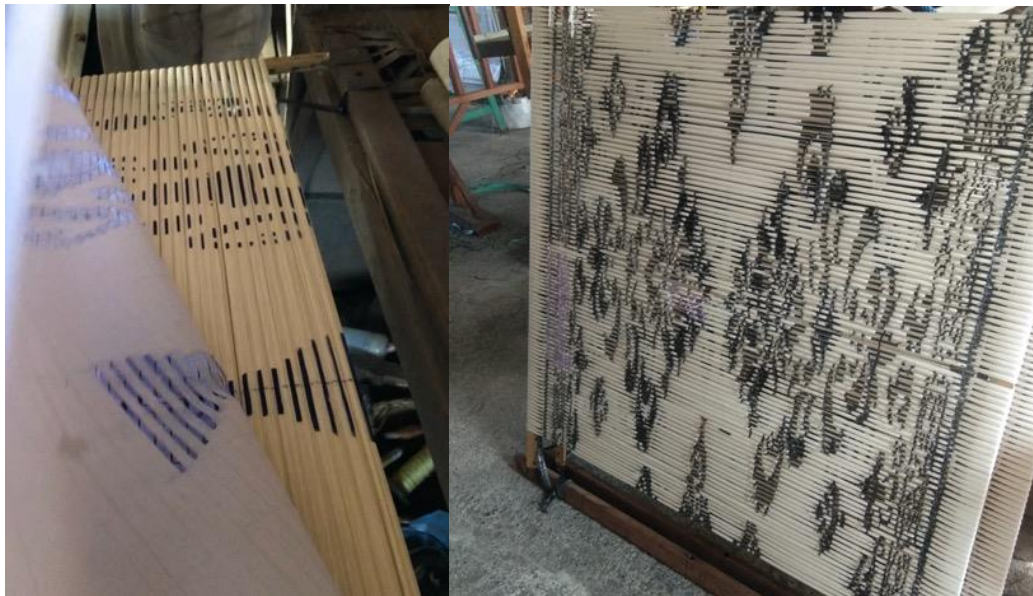
Figure 5. (a) left: the weft threads frame that have been patterned; (b) right: the weft threads frame that the patterns have been tied
