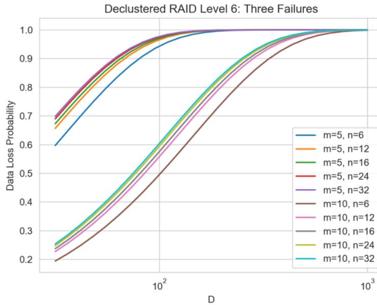
**Figure 5.** Dataloss probability in the presence of three failed disks in a declustered RAID Level 6 with  $m$  stripes and  $n$  data disks per stripe in dependence on  $D$ , the number of disklets per disk
