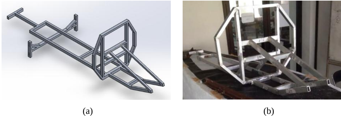
Figure 2. (a) Chassis prototype design and (b) after fabricated construction
